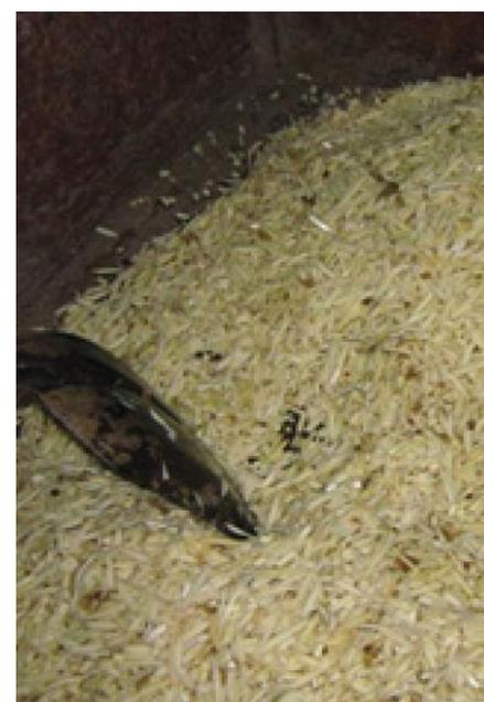
*Original speed setting and bar spacing removed fries and cuttings*
