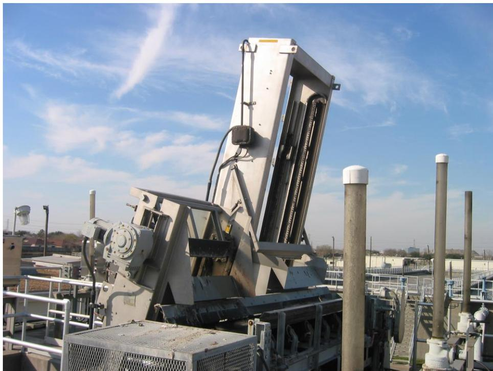
*The MS Bar Screen operated for 10 years of run time with no chain, sprockets, or lower bearings requiring replacement*
